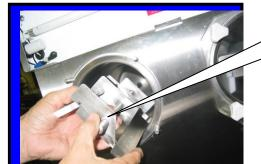
Step 7: Install beater bar assembly C6530 into cylinder.
