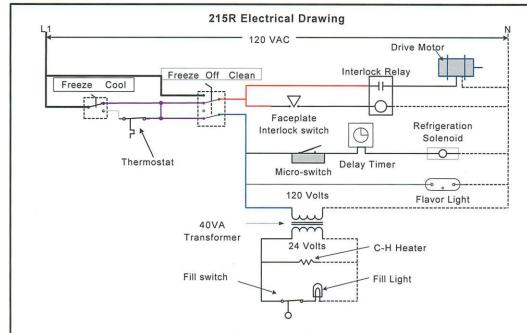
Note: Schematic is for either side of the dual machine.
