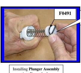
Install **O-rings** onto plunger
