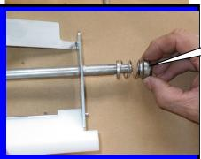
Step 5: Install spring seal **F0355**
