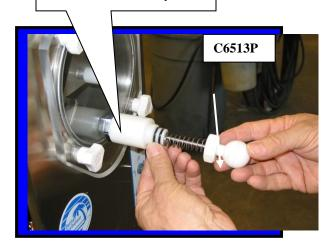
Installing Faceplate onto front of Machine.
