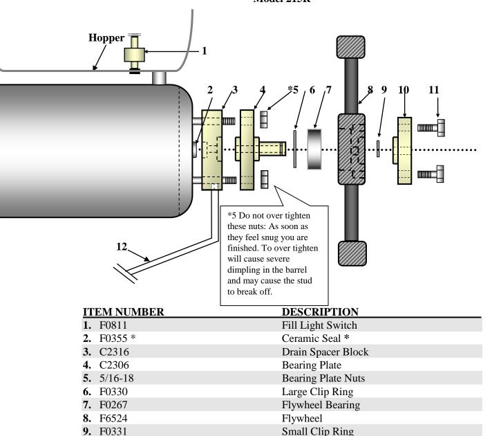
\*Note: F0355 is the part number for the <u>Spring Seal Assembly</u> Which includes the ceramic seal (No.2 above)
