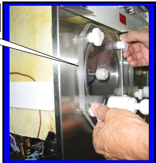
Installing faceplate C6521 onto front of Machine.
