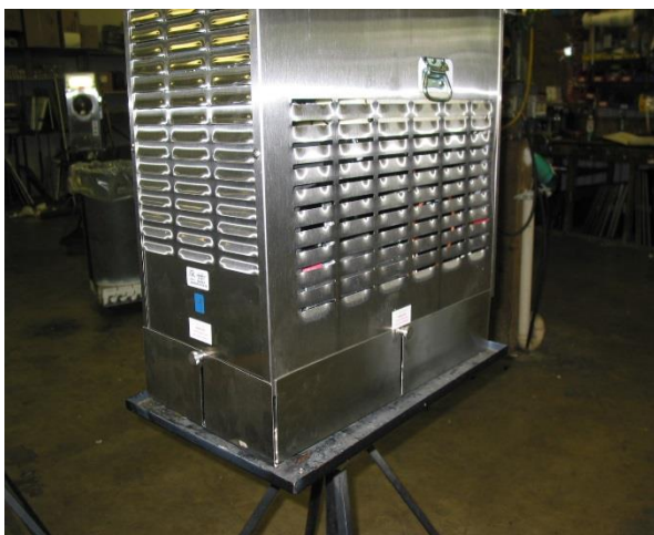
Skirts down for operation. For normal operation/freezing mode.
