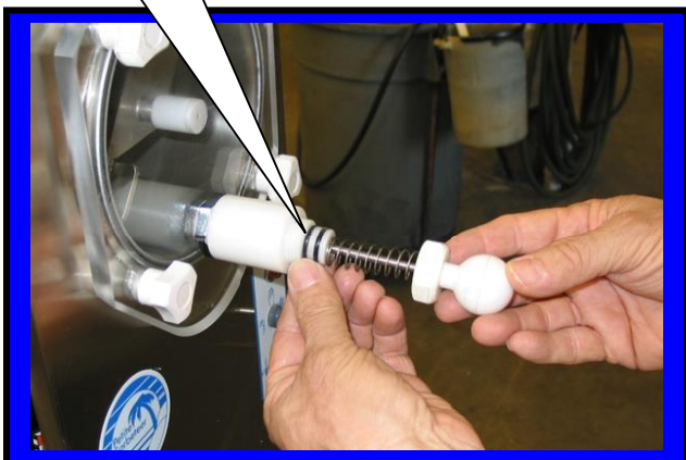
Installing Plunger assembly C6513P into faucet body
