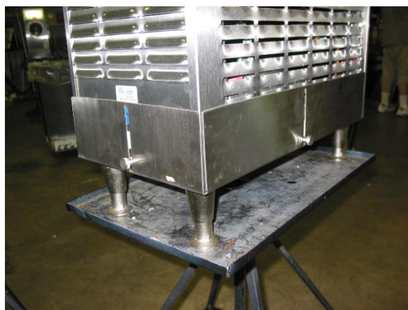
Skirts down for operation. For normal operation/freezing mode.
